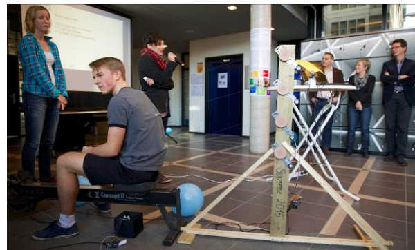
Figure 4. Project result: a device to measure the rower's back angle
