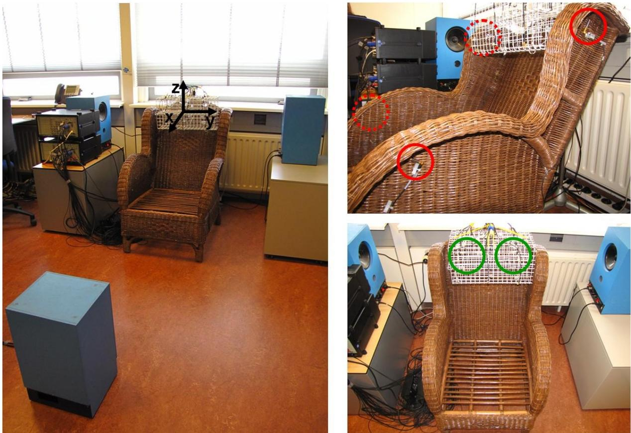
Figure 1: 'Silent Chair' experimental setup. The red circles show the physical locations, the green circles the virtual locations. The primary source is placed in front of the chair, the two secondary sources on the sides.
