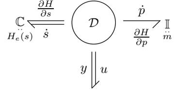
Fig. 1. Generalized model of a variable stiffness actuator with a load - The internal elastic elements are represented by the multidimensional  $\mathbb{C}$ -element, and the load is represented by the  $\mathbb{I}$ -element. The internal degrees of freedom are actuated via the control port  $(u, y)$ .
