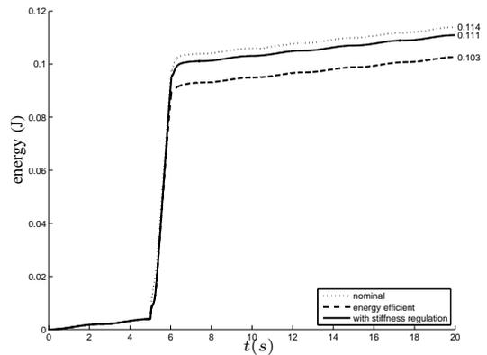
Fig. 2. Energy supplied via the control port - The energy efficient control law clearly achieves a reduction in supplied energy. When stiffness regulation is added, some of the gain in efficiency is lost.
