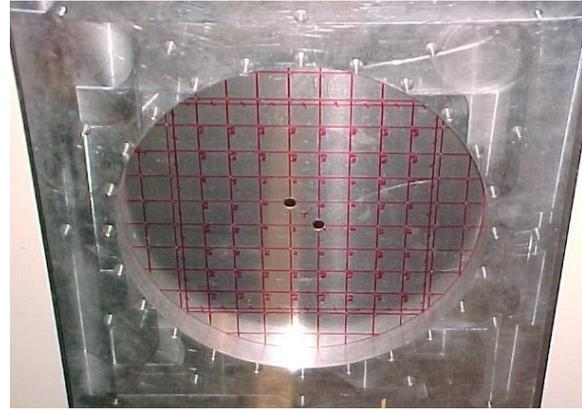
Figure 9: Aluminum panel with 2 holes, with markings for the remaining holes to be drilled.
