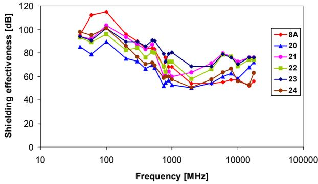
Figure 6: Shielding effectiveness of several GRP panels
