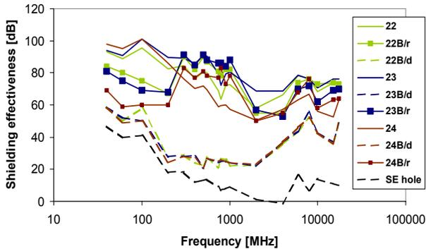
Figure 8: Shielding effectiveness of several GRP panels, before damage, after damage and after repair
