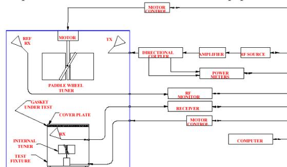
Figure 4: Nested Chamber method as described in [15](details of the text can be found in [15])
