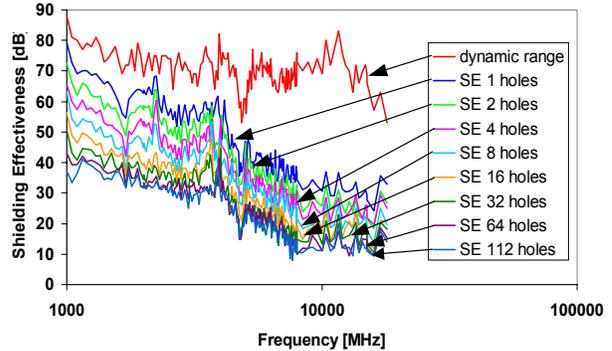
Figure 10: Shielding effectiveness of panel with holes
