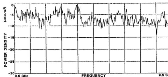
Figure 3: Power density inside reverberation chamber when the mode stirrer rotates
