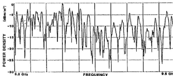
Figure 2: Power density inside reverberation chamber when the mode stirrer does not rotate
