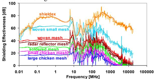
Figure 12: SE of various wire mesh
