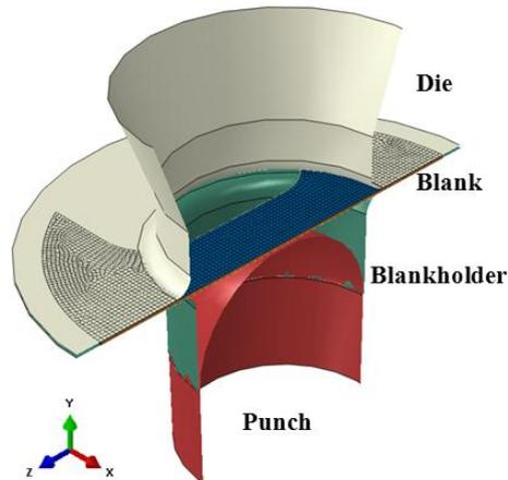
Figure 2; FEM Schematic of Nakazima test.
