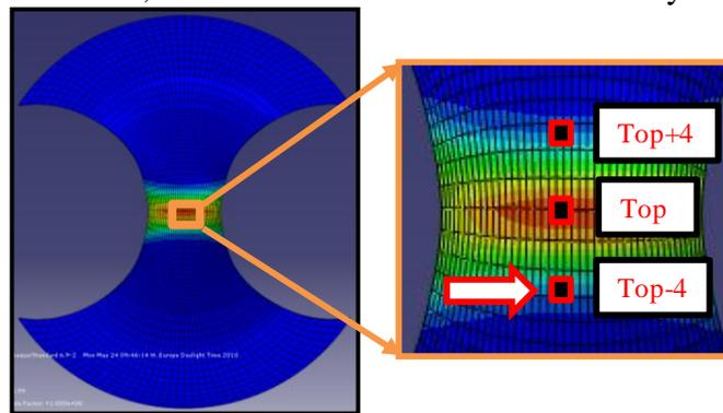
Figure 3; Schematic of elements selection for strain rate localization.
