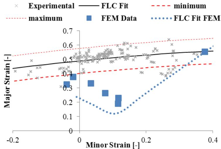
Figure 7; FLC experimental and FEM results for DP600 and 20 mm punch.
