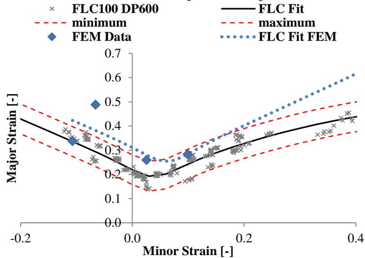
Figure 5; FLC experimental and FEM results for DP600 and 100 mm punch.
