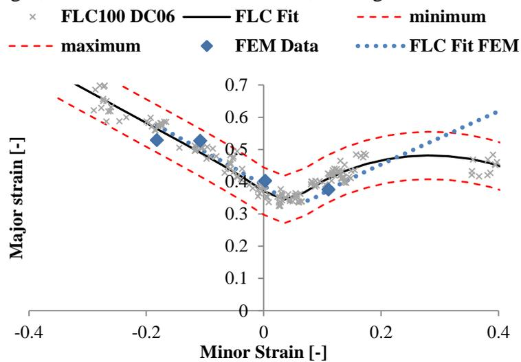
Figure 4; FLC experimental and FEM results for DC06 and 100 mm punch.
