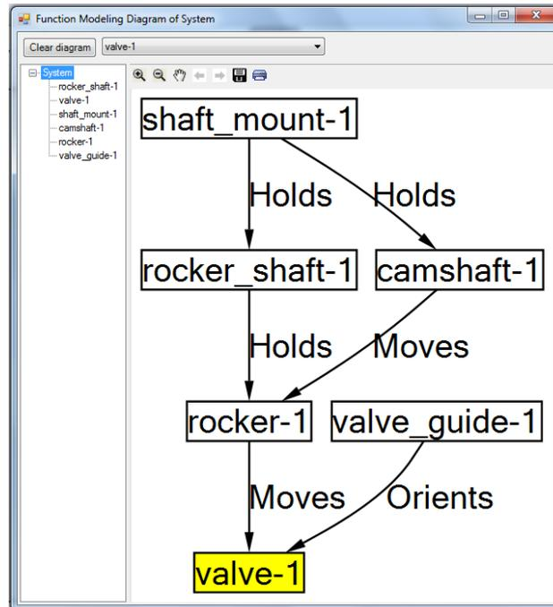
Fig. 3. Function Model diagram
