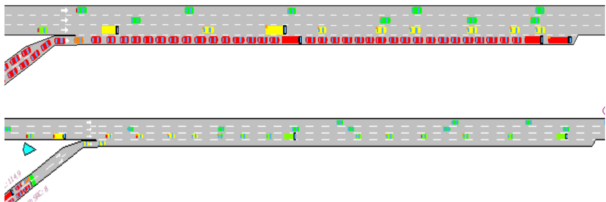
Figure 7 – Merging behavior before (above) and after (below) model calibration
