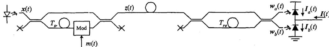
Figure 1: A conventional Coherence Multiplexing System
