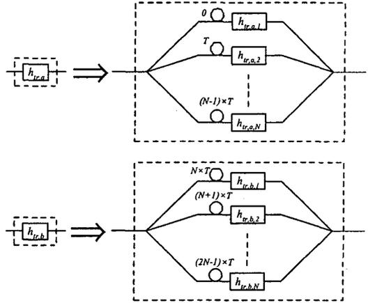
Figure 3: Substitution of transmitter filters
