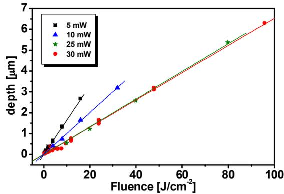
Fig. 2: Graph of the laser tracks depth dependence on used fluence. The four lines belong to four different laser average powers 5, 10, 25 and 30 mW.
