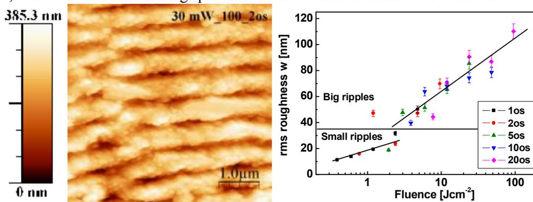
Fig. 3: Example of AFM scan performed on the laser treated sample at 30 mW laser pulse power, 100 mm/s machining velocity and 2 overscans. The right graph of RMS roughness dependence on the used fluence shows 25 values in different colours according number of overscans. The graph is divided into two regions corresponding to small and big ripples induced roughness.
