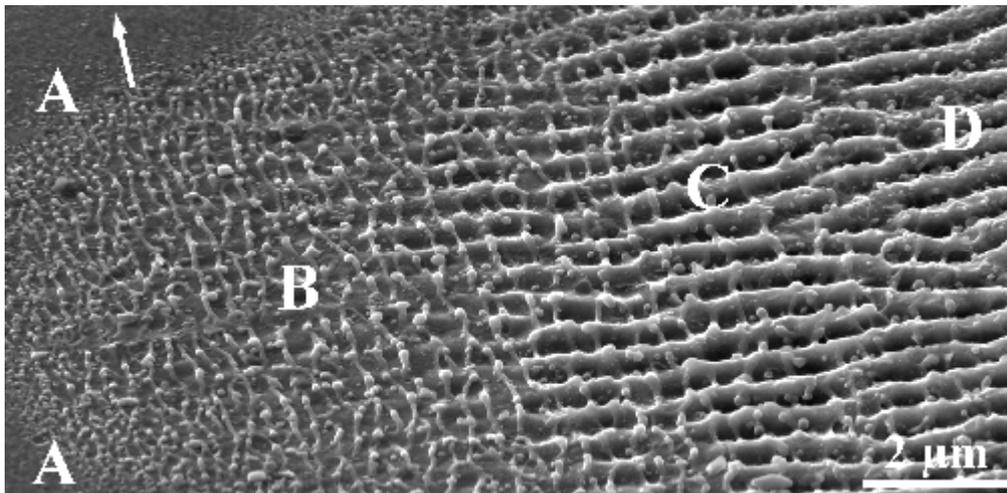
**Fig. 1** The end of the track illuminated by a few last pulses from the whole 500  $\mu\text{m}$  long laser track (horizontal to the SEM picture, machined from right to left) which was created by 30 mW average laser power. Repetition rate of 50 kHz and machining speed of 50 mm/s results in 1  $\mu\text{m}$  distance between subsequent pulses. The view is 55° inclined from normal to the sample surface. The beam polarization vector is marked by arrow.
