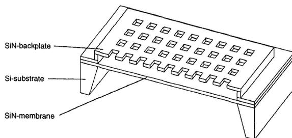
Figure 1: A silicon condenser microphone [1].
