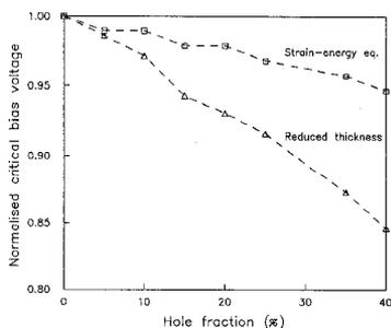
Figure 5: Normalised critical bias voltage for a microphone with the SE- and RT backplate model.
