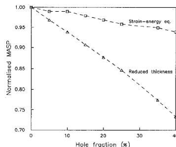
Figure 6: Normalised maximum allowable sound pressure for a microphone with the SE- and RT backplate model.
