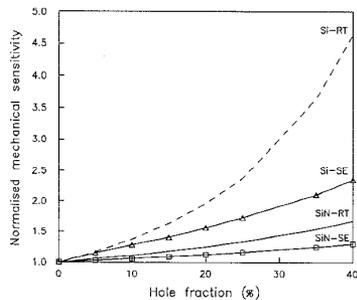
Figure 4: Normalised mechanical sensitivity for two perforated plates.
