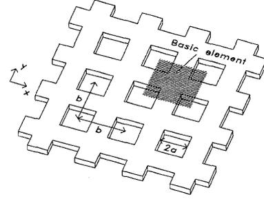
Figure 2: Perforated plate with square holes in a regular pattern.
