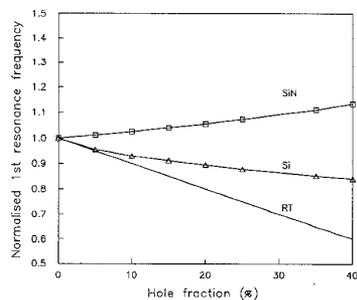
Figure 3: Normalised first resonance frequency for two perforated plates.
