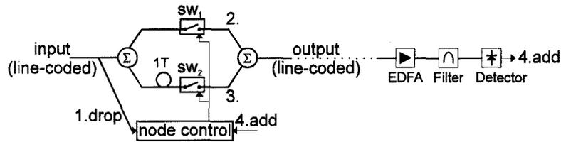
**Figure 3: minimal ADM configuration for OOK operation.**
