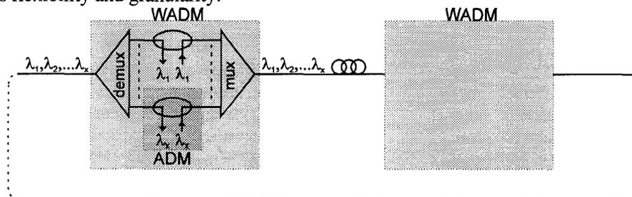
**Figure 1: Situation of WADM and ADM in a ring network topology.**
