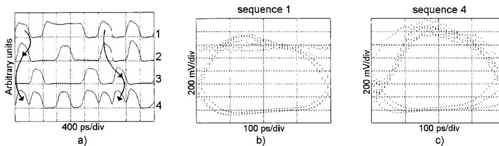
**Figure 4:** a.) 1. the 'drop' sequence; 2. the output of switch-1; 3. the output of switch-2; 4. the 'add' sequence (numbers refer to Figure 3). b.) eye diagram of sequence 1 (@ -32 dBm). c.) eye diagram of sequence 4 (@ -32 dBm).
