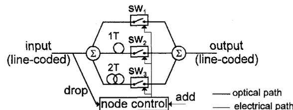
**Figure 2: wavelength- and modulation format independent ADM**
