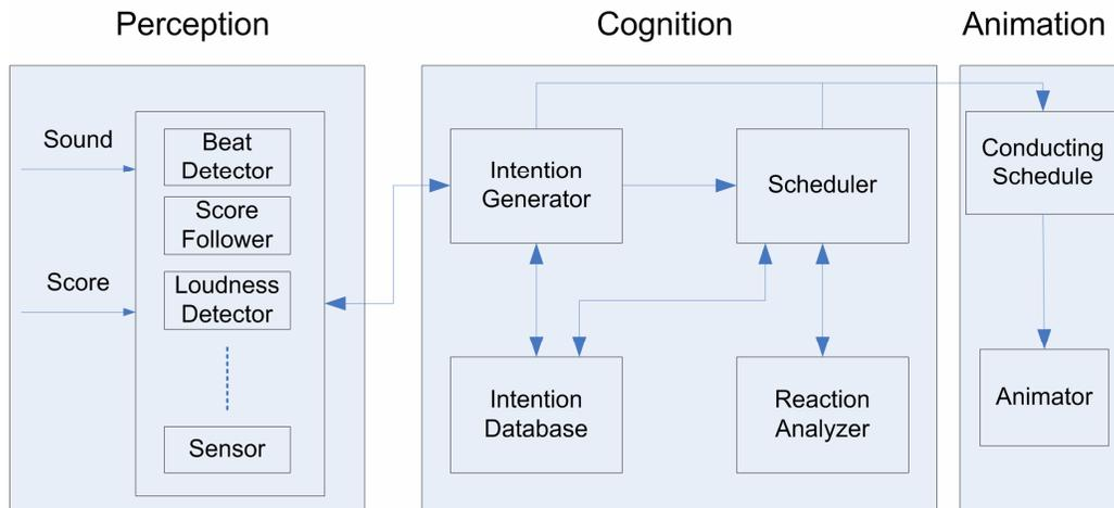
**Figure 2. Global architecture of the Virtual Conductor**
