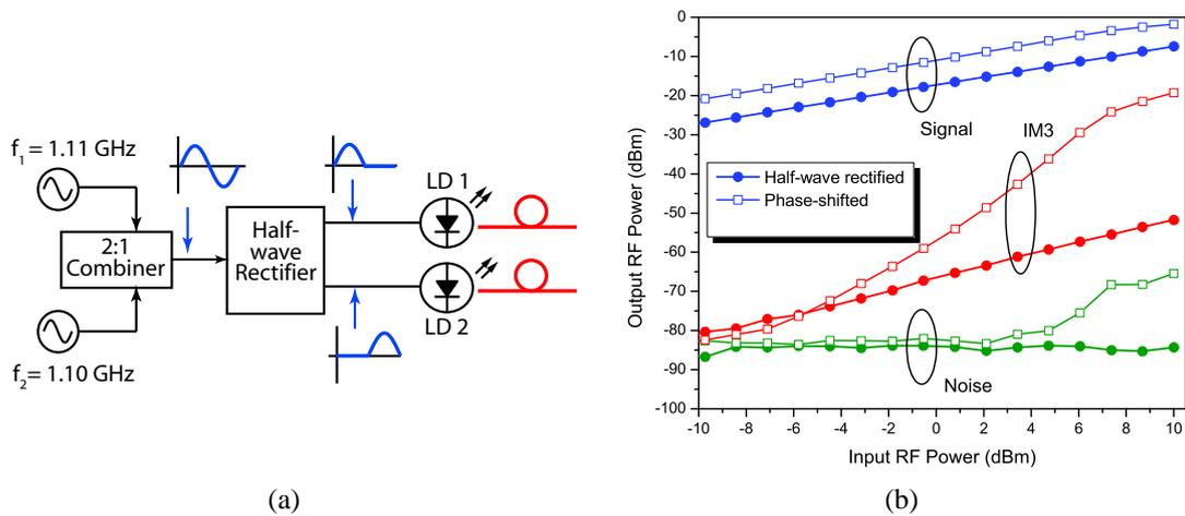
Figure 4: (a) External half-wave rectification prior to the optical modulations. (b) Comparison of noise and distortion in the BMD link with the phase shift method and with the external half-wave rectification.
