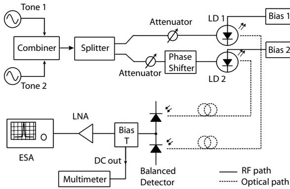
Figure 1: Measurement setup of the BMD link
