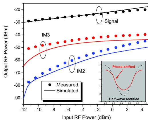
Figure 3: Intermodulation distortion in the BMD link. The lasers are biased at 10 mA.
