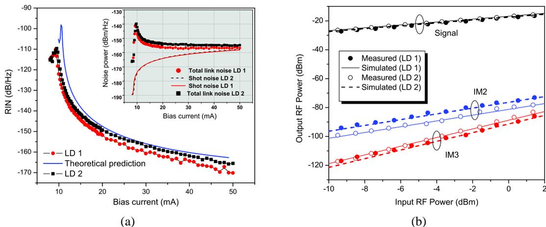
Figure 2: Laser characterization. (a) RIN as a function of the bias current. Inset : the measured total link noise as a function of the bias current (b) Intermodulation distortion
