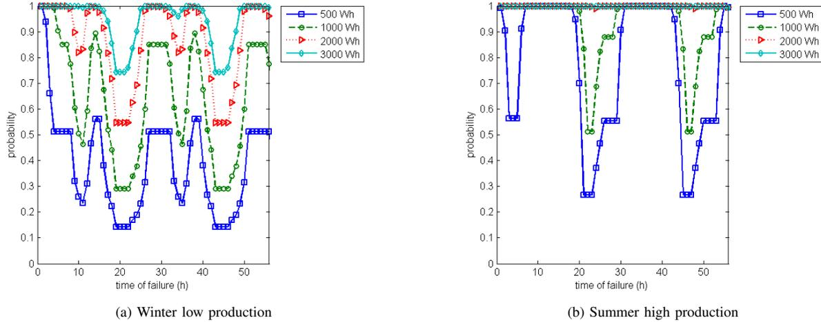
Fig. 12. Probability of surviving a grid failure as function of the time that the failure occurs for the *Smart* strategy. The following two scenarios are considered, (a) winter day with low production, and (b) summer day with high production.
