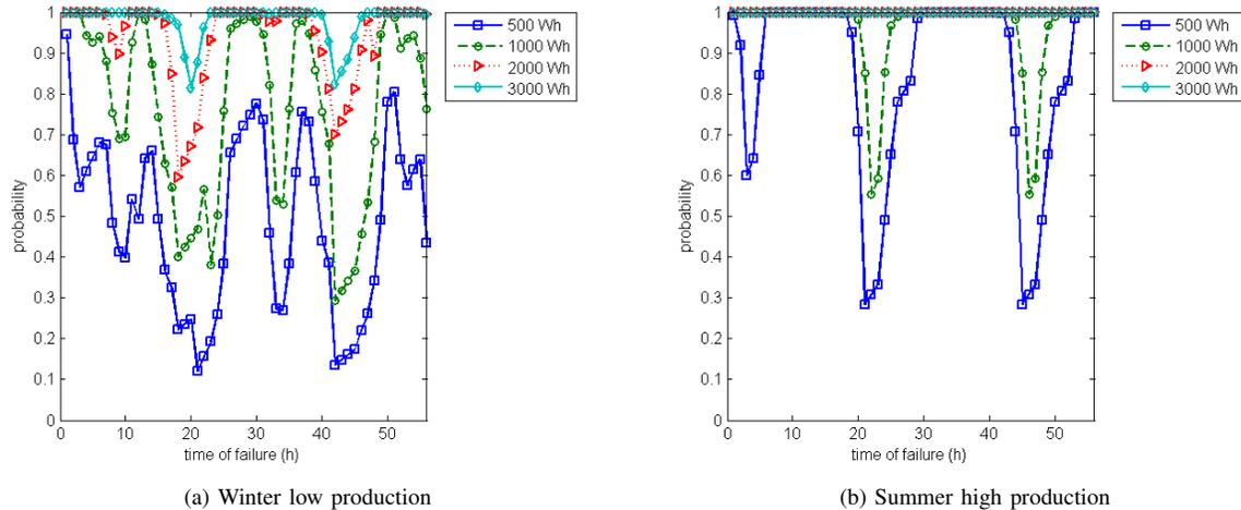
Fig. 13. Probability of surviving a grid failure as function of the time that the failure occurs for the *Conservative* strategy. The following two scenarios are considered, (a) winter day with low production, and (b) summer day with high production.
