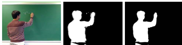
Figure 2. (a) Original video frame (b) Segmented foreground object (c) Frame after morphological operations and smoothing.
