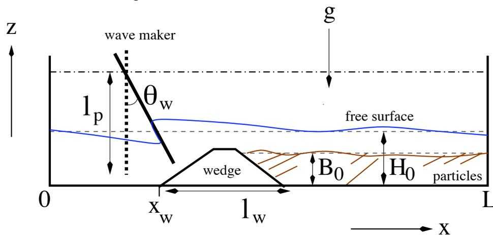
Figure 1. Sketch of the Hele-Shaw cell from the side with the wedge, waterline, particle bottom, and wave-maker rod in two positions outlined. The wedge holds particles away from the wave maker.
