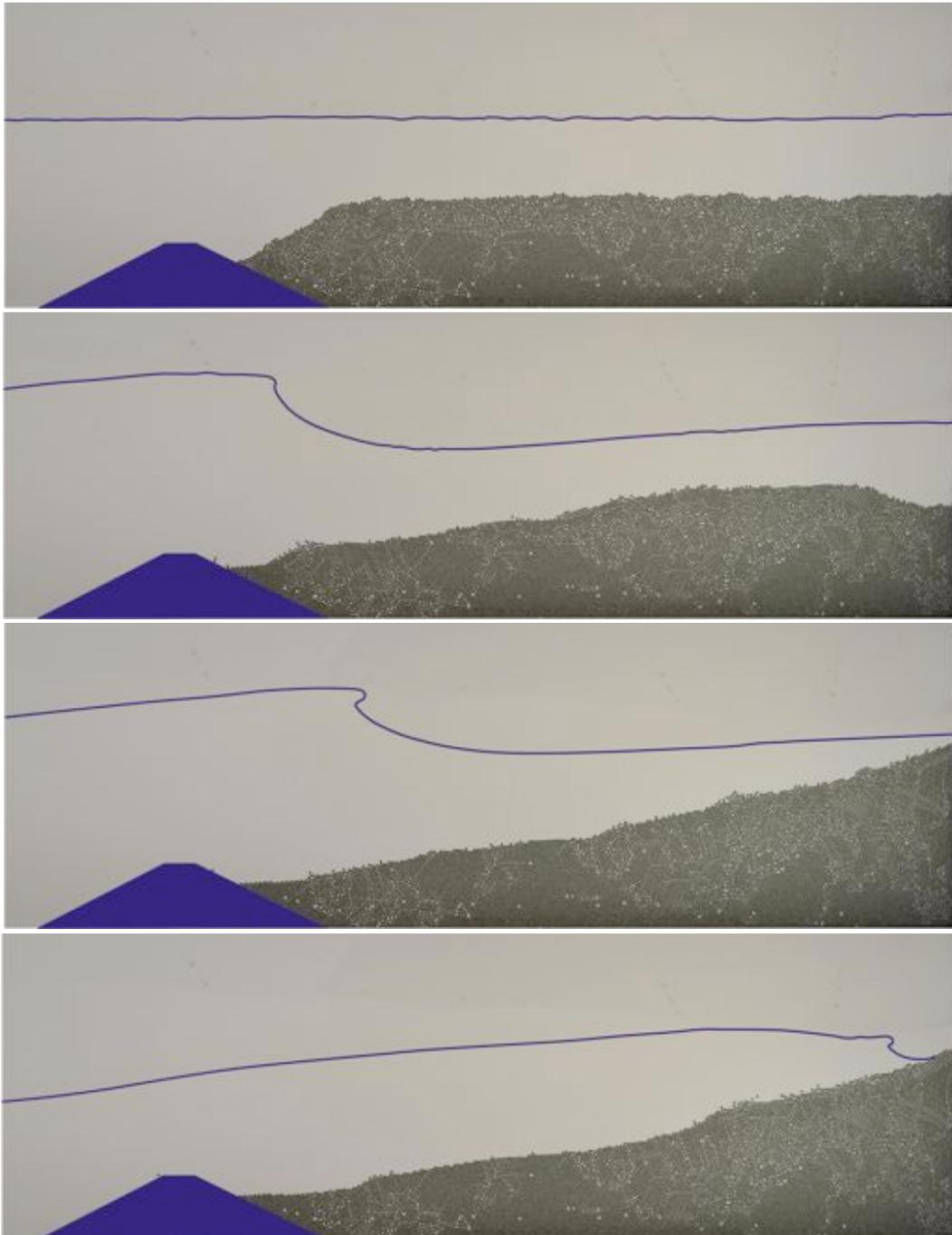
Figure 4. Profiles at  $t = 0, 5, 21, 20, 28, 50 \text{ min}$  (top to bottom) show beach formation under impact by monochromatic waves. Initially, waves move material from near the wedge to the shore. On longer time-scales a beach of nearly constant slope forms at the right wall, where a beach arises (last image).
