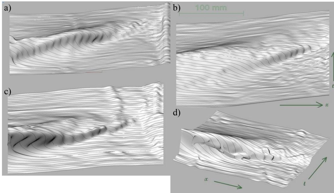
Figure 3. Rendered graphics of measured water surfaces versus space  $x$  (on the same scale) and time  $t$  are given for the (four) breaker types: a) spilling breaker (beach grains visible on right), b) surging breaker, c) collapsing breaker (beach grains visible on right and upper right), and d) plunging breaker. Time between frames is 0.02s.
