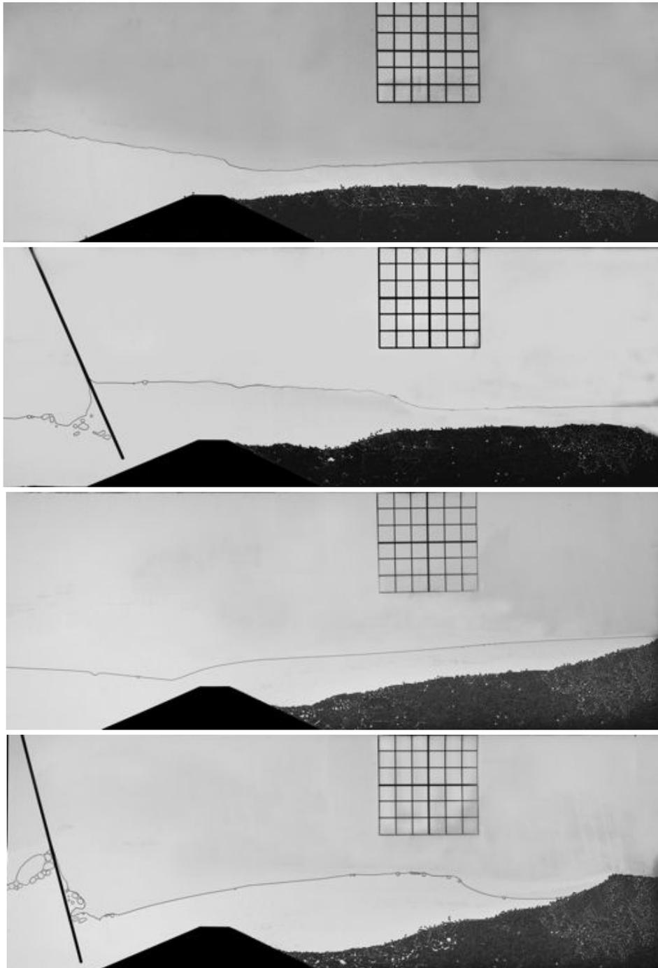
Figure 5. Profiles (top to bottom) are shown of beach formation under wave impact for two wave frequencies, changed intermittently, at  $t = 0, 2.5, 10.5, 25.5$ min.
