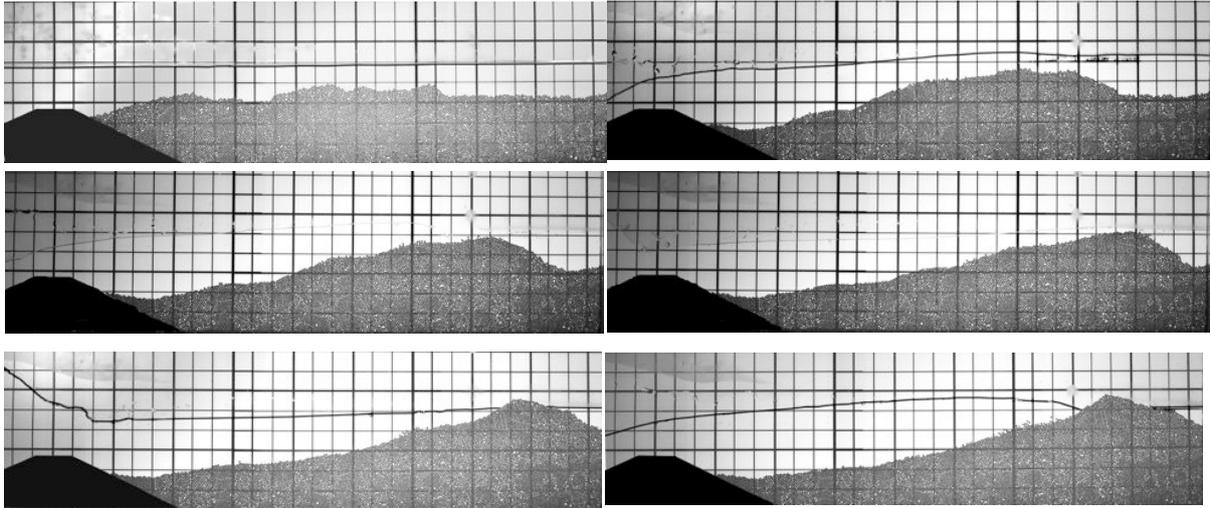
Figure 6. Snapshots are shown at  $t = 0, 9, 18, 27, 36$  and  $45$  min. (top to bottom) showing dune formation. A waterline separates water from air. We intermittently change wave frequencies between  $0.6$  and  $0.9$  Hz. Finally, a quiescent lake emerges behind the dune (last image).
