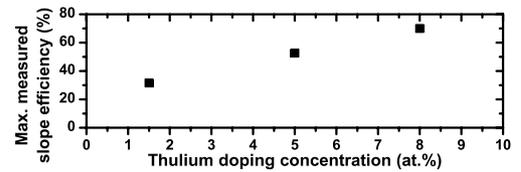
Fig. 2. Maximum measured slope efficiencies for thulium-doped monoclinic double tungstate channel waveguide lasers with different doping levels.
