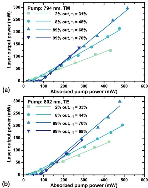
Fig. 1. Output power versus absorbed pump power of a 8at.% thulium-doped channel waveguide laser pumped at (a) 794 nm in TM polarization and (b) 802 nm in TE polarization.
