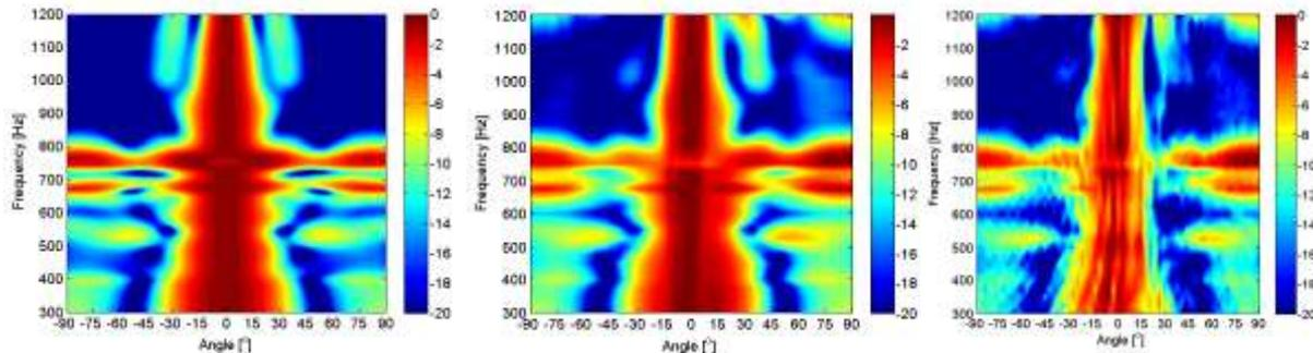
Fig. 12. Impact of road surface impedance and nearby scattering objects on beam forming performance: (left) reference configuration, (middle) impact of 20m long asphalt road, (right) impact of asphalt road and parked cars
