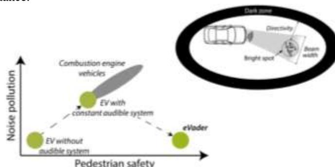
Fig. 2: eVADER approach using a directional acoustic warning system.
