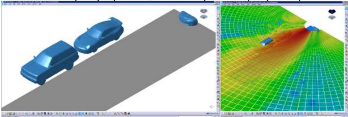
Fig. 11. Impact of road surface impedance and nearby scattering objects on beam forming performance: (left) H-matrix BEM model discretisation, (right) spatial distribution of the acoustic pressure field at 600Hz
