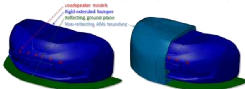
Fig. 8. FEM-AML model of the warning signal generator integrated into the front bumper
