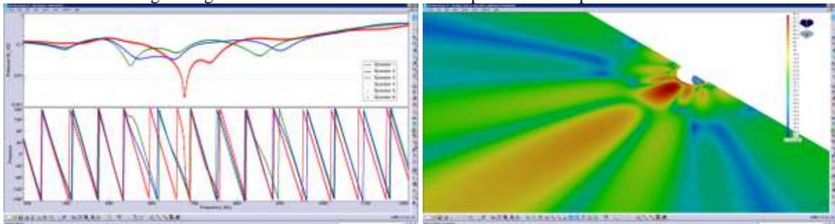
Fig. 9. Acoustic pressure responses obtained with the baseline FEM-AML model: (left) individual acoustic transfer functions for the six speakers, (right) forward-facing acoustic beam at 900Hz
