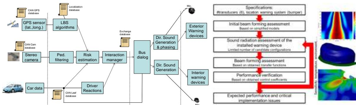
Fig. 1. Overall eVADER warning system layout (left) and exterior warning device design strategy (right)
