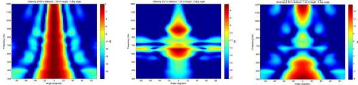
Fig. 6: Beam shapes for more realistic car geometry with reflecting ground surface; steering at an angle of 0 degrees. Beam optimisation at 40m distance, beam evaluation at 40 m distance (left), beam optimisation at 5m distance, beam evaluation at 40m distance (middle), beam optimisation at 40m distance, beam evaluation at 5m distance (right).
