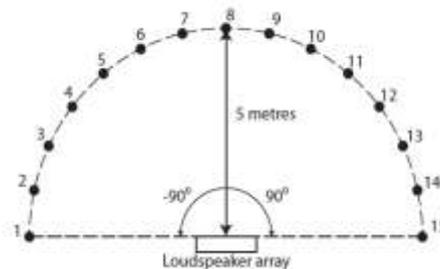
Fig. 5: Example configuration used to define the beam former showing the loudspeaker array and a number of microphones on a circle, in this case using 15 microphones at a distance of 5m from the centre of the array.
