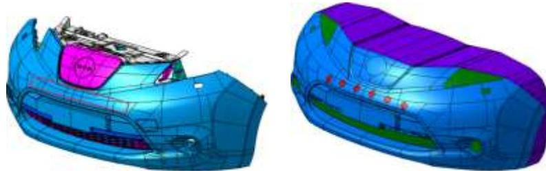
Fig. 7. Original (left) and computational (right) bumper geometry
