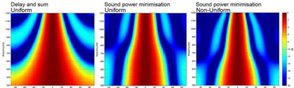
Fig. 3: Sound pressure level in dB relative to the sound pressure level in the main beam (steering at 0°) for an array of 6 point sources using uniform and non-uniform array geometries and Delay and sum and sound power minimisation strategies.
