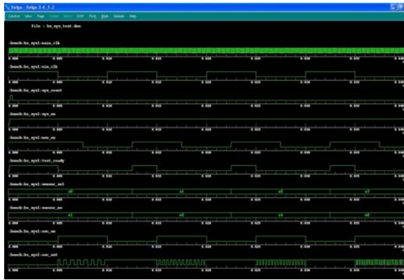
Figure 12. VHDL-AMS simulation result of the oscillation-based DNA sensor array. The last signal shows the oscillation frequency in the previous situations (Fig. 4).
