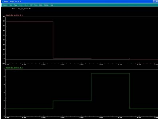
Figure 4. VHDL-AMS simulation input ( \epsilon_r and t_{ox} ) in the case of a bare Au electrode, functionalization, DNA hybridization and failure.
