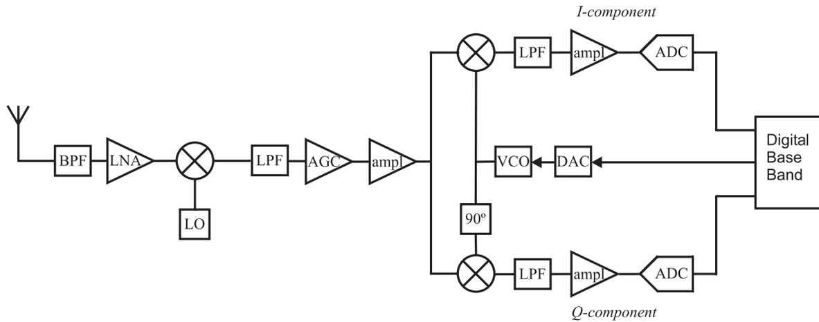
**Figure 1: Conventional heterodyne receiver.**
