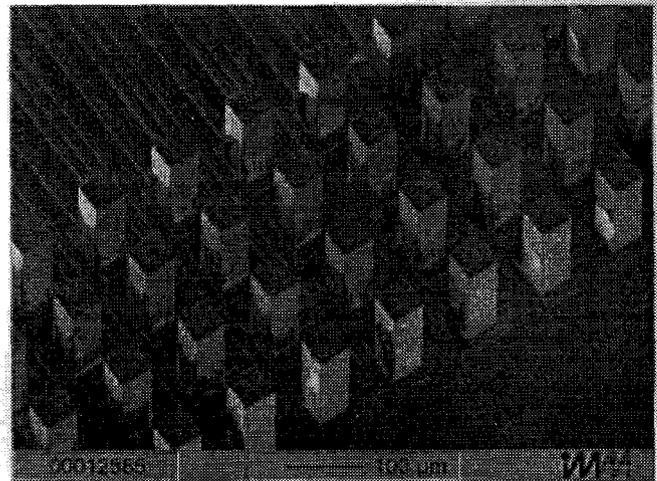
Figure 4 Array with 200  $\mu\text{m}$  tall needles, realized with aligned x-ray lithography (LIGA) on silicon substrate with 8  $\mu\text{m}$  Cu interconnection wiring.
