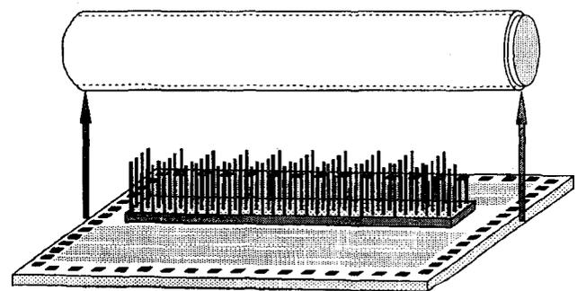
Figure 2. Schematic overview of a CMOS chip carrying a 3D array of 128 microelectrodes, to be inserted into a nerve. For dimensions, see Fig. 3.
