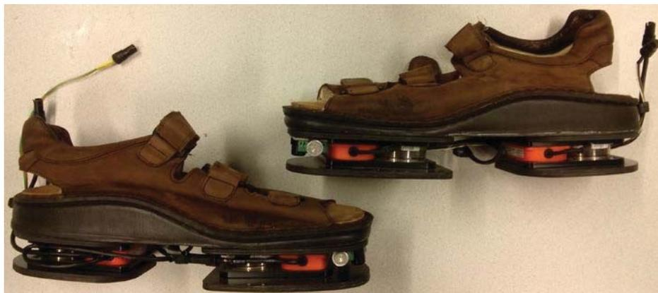
Figure 1. Xsens ForceShoes™ containing two inertial and two force/moment sensors. Near the inertial sensor in the forefeet an ultrasound transducer is mounted in each shoe.
