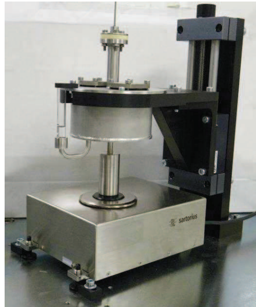
Figure 5: Weighing cell, reservoir and moisture saturator for the line n°2 (10 ml.h -1 to 100 ml.h -1 ).
