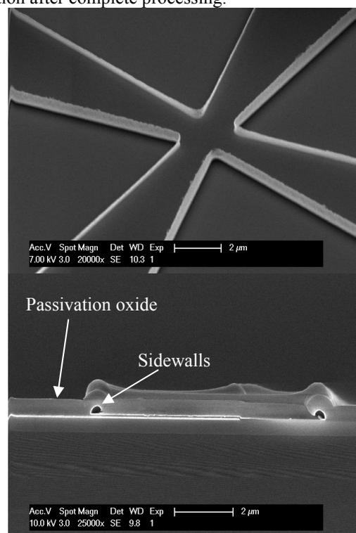
Figure 1: Standing sidewalls formed due to re-deposition; (a) after resist removal, (b) bad coverage of passivation layer after complete processing
