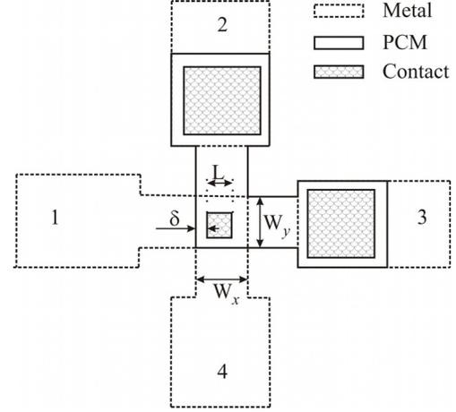
Figure 3: Cross Bridge Kelvin Resistor structure showing upper (PCM) layer, lower (metal) layer and the contact structure ( $\delta$ ,  $L$ )
