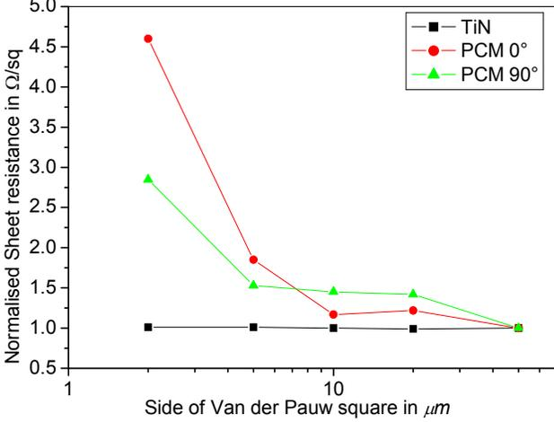
Figure 2: Sheet resistance measurements on PCM Van der Pauw structures with standing sidewalls, measured in two different directions with 90° rotation. The normalized TiN results (no sidewalls) are shown for reference.
