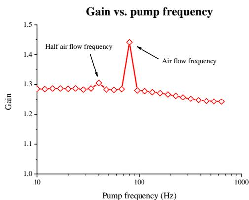
Figure 9: Gain vs. pump frequency  $f_p$ .
