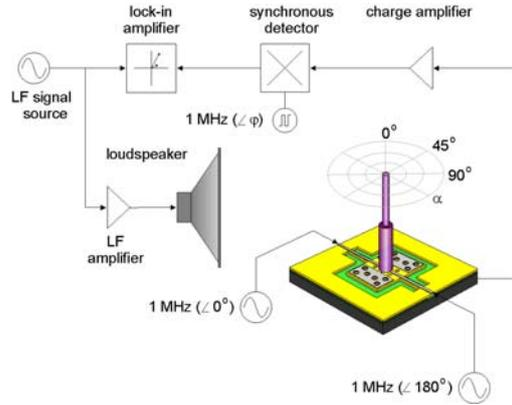
Figure 2: Performing flow measurements with artificial hair-sensors.
