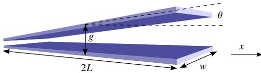
Figure 5: Tilted rectangular capacitor.
