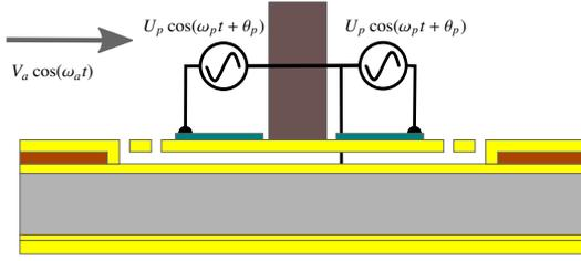
Figure 4: Modulating the torsional spring stiffness in time.
