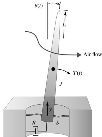
Figure 3: Model of a flow sensing hair [5].
