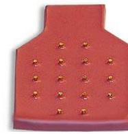
Figure 1. 2D-electrode array that was used for the recordings (Helmholtz Institute, Aachen, Germany). The array was placed on the biceps brachii with the columns parallel to the line from the acromion to the cubital fossa.
