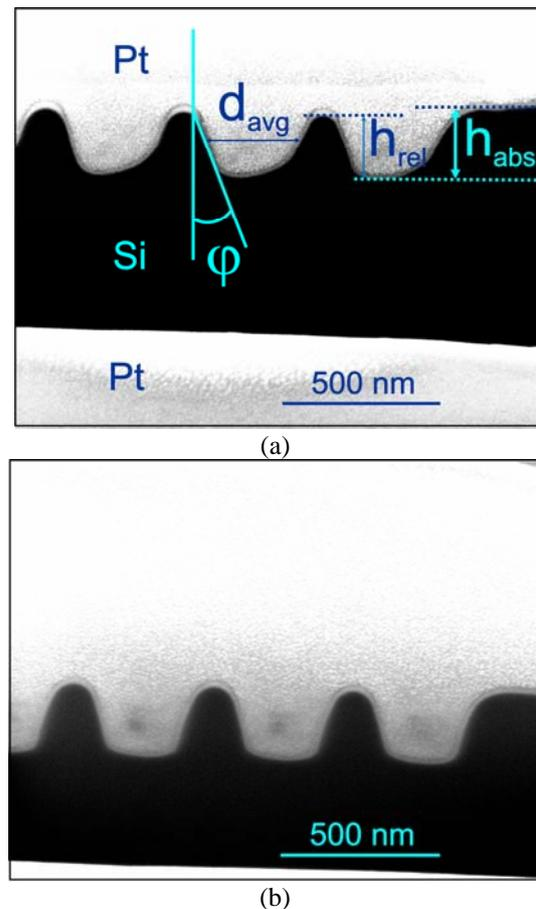
**Fig. 3:** Patterns milled at 48 pA using 12 loops and a dwell time per pixel of 0.1 ms. (a) Raster scan (b) Spiral scan.
