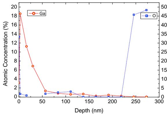
**Fig. 5:** Depth variation of gallium and oxygen atomic concentrations through SOI as measured by XPS.
