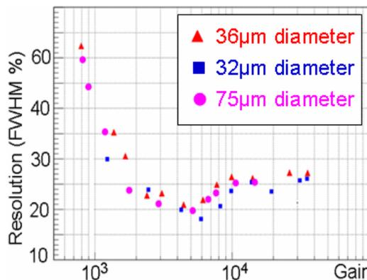
Figure 7: Resolution vs. gain for various hole diameters.
