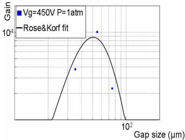
Figure 3: Gain at 450 V on the grid for various gap thicknesses. The data points are fitted using the Rose and Korff formula.
