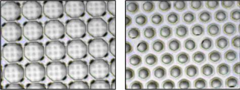
Figure 1: A 80- $\mu\text{m}$  hole pitch, 75- $\mu\text{m}$  gap InGrid, showing 10% gain homogeneity (left side) and a 60- $\mu\text{m}$  hole pitch, 35- $\mu\text{m}$  gap InGrid exhibiting 1.6 % gain homogeneity with a 240  $\mu\text{m}$  pillar pitch (right side)
