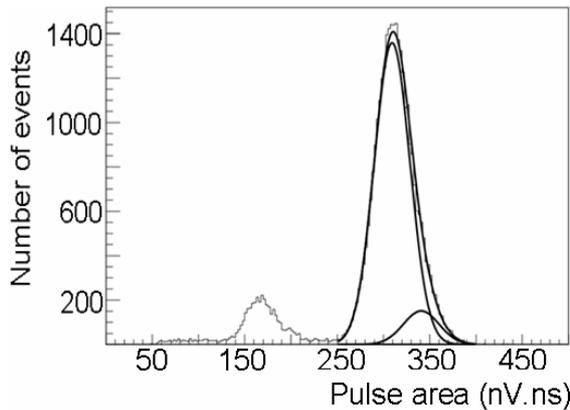
Figure 6:  $^{55}\text{Fe}$  spectra in Argon showing the fit of the 5.9 keV and 6.5 keV lines.
