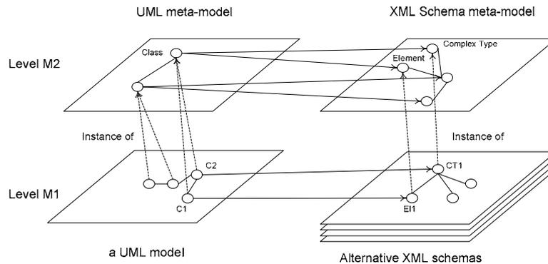
Figure 2: Multiple alternative transformations for a given UML class model into XML schemas.
