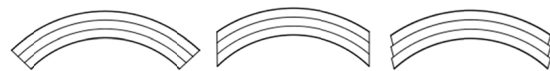
Fig.6 Kirchhoff bending (left), with intra ply shear (middle) and a combination with inter-ply shear (right).
