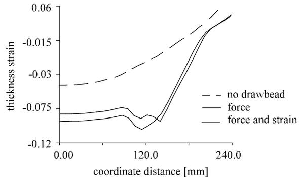
FIGURE 13. THICKNESS STRAIN DISTRIBUTION RECTANGULAR PRODUCT.
