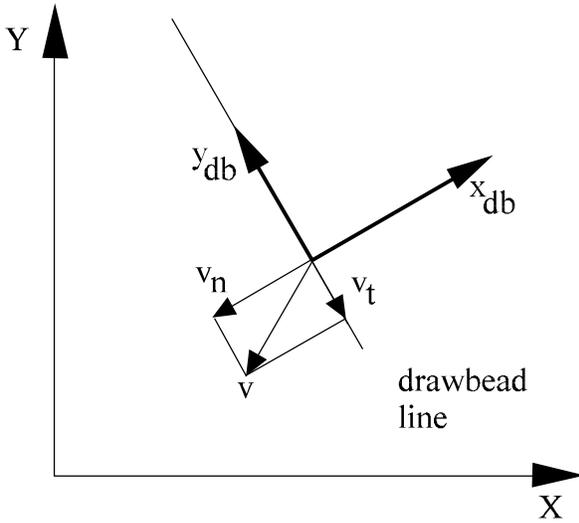
FIGURE 4. DRAWBEAD COORDINATE SYSTEM
