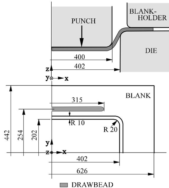
FIGURE 11. BLANK AND TOOL GEOMETRY OF THE RECTANGULAR PRODUCT
