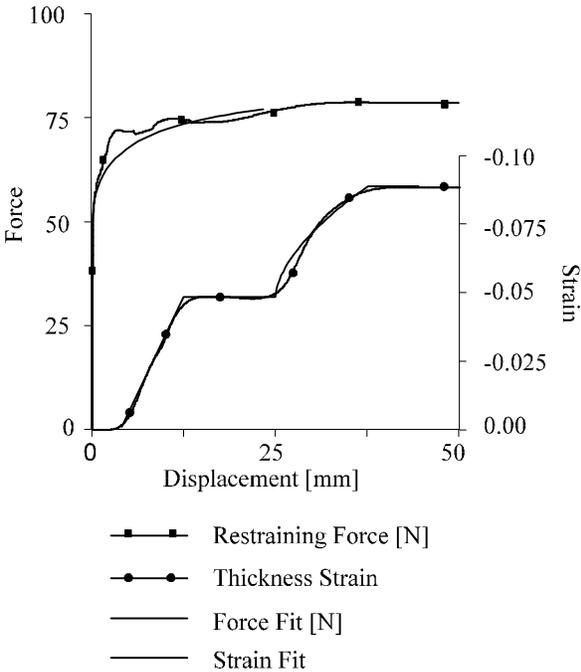
FIGURE 5. DRAWBEAD FORCE FIT AND STRAIN FIT
