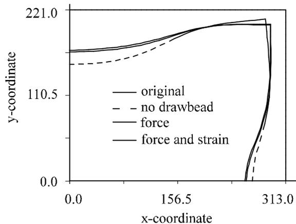
FIGURE 12. FLANGE SHAPES OF THE DIFFERENT SIMULATIONS OF THE RECTANGULAR PRODUCT.
