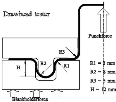
FIGURE 1. EXPERIMENTAL SET-UP OF THE DRAWBEAD TESTER
