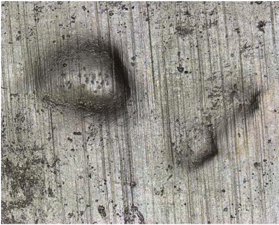
(c) Devulcanized material, amplification 50*; surface 2*2 mm 2 .
