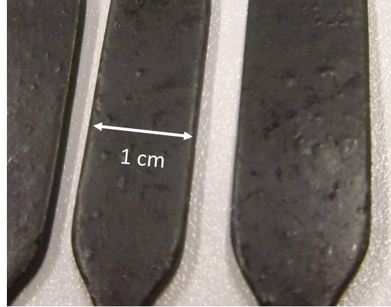
(b) Devulcanized material mixed with 50/50 %wt virgin rubber; visible particles.
