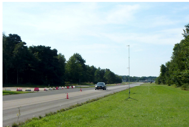
Figure 6 – Test area at airport Twente, photo taken during pass-by measurements.
