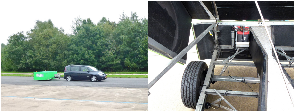
Figure 13 – Closed CPX trailer, padded with foam.
