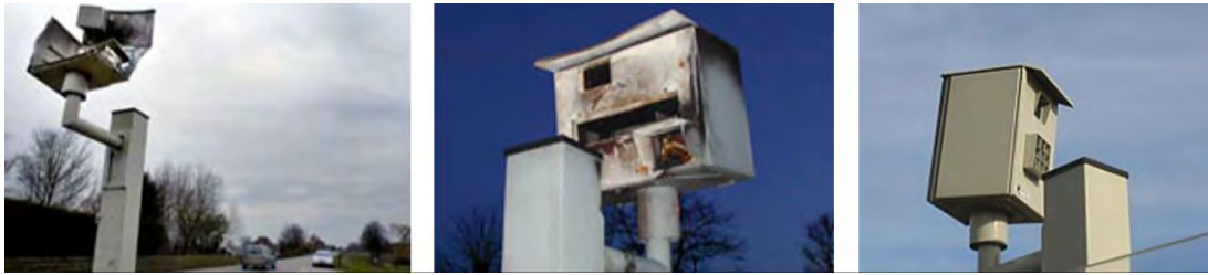
Figure.2 Molested speeding camera's in the Netherlands (left and mid) and their typical design (right).
