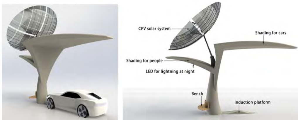
Figure 11. ‘Tulip’ concept for an electric vehicle charger station, developed by Jorien Bootsvelde and Katja Schuitemaker.
