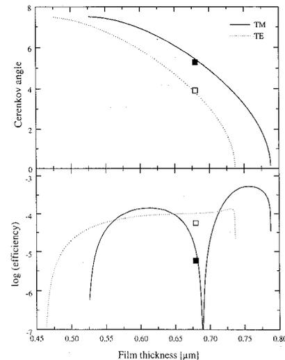
**CWL6 Fig. 2.** Measured and theoretically calculated Cerenkov angle and second-harmonic efficiency from the corona-poled thin film.  $\lambda = 1064 \text{ nm}$ .
