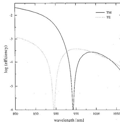
**CWL6 Fig. 3.** Cerenkov second-harmonic efficiency predicted by coupled mode theory vs fundamental wavelength. Film thickness is 550 nm.
