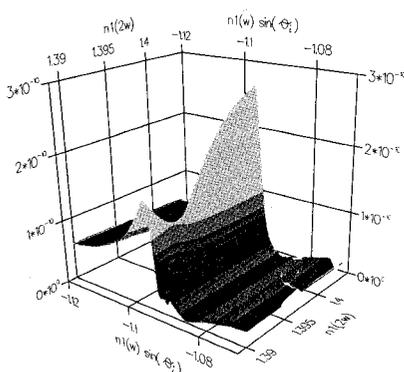
**CWL5 Fig. 2.** The amplitude of the nonlinear reflected signal for a system of Fig. 1.  $n_1(\omega) = 1.534$ , sinusoidal corrugation with  $d = 4 \mu\text{m}$  and  $h = 15.4 \text{ nm}$ . TM polarized light with pump wavelength  $1.06 \mu\text{m}$ .  $\chi_{xxx} = \epsilon_0$ ,  $\chi_{yyy} = 0$ .  $t = 0.01 \mu\text{m}$ .
