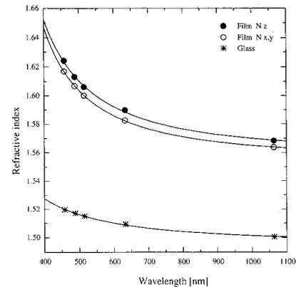
**CWL6 Fig. 1.** Refractive indices and birefringence of the 78 wt. % nitro-calix[4]arenes—PPMA thin film after corona poling and of the glass substrate.
