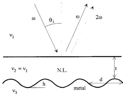
**CWL5 Fig. 1.** Schematic representation of corrugated nonlinear system. The nonlinear media extends from the grating surface to a plane at distance  $t$  from the groove top. The cladding and the nonlinear layer indices are equal. The metal is silver.
