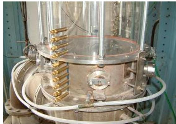
Fig. 2. Flow sheet of the fluidized bed (top) and close-up of the bottom section of the fluidized bed, showing the positions of the measurement probes (bottom)
