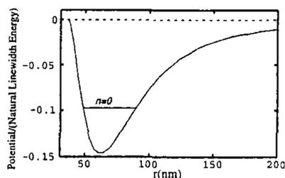
QMF5 Fig. 3. Calculated trap potential as a function of the distance from the surface of the tip. The potential is normalized by the natural linewidth energy of a Rb atom.
