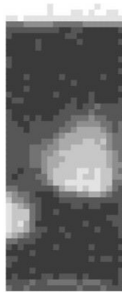
Figure 10: Snapshot of the bed porosity in the case where two bubbles are present. The lower bubble sticks to the wall and is much more asymmetric than the bubble in the core of the bed.
