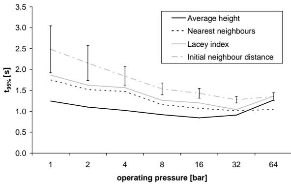
**Figure 11:** The 95% mixing time versus operating pressure for four different methods. For the initial neighbour distance method the error margins are shown.
