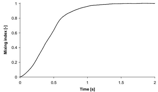
**Figure 3:** Mixing index determined with the neighbour distance method, calculated with the data from Figure 2.
