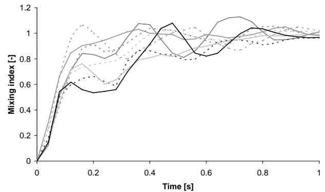
**Figure 10:** The mixing index calculated with the sphere radius method for 8 parts of the simulation at an operational pressure of 8 bar.
