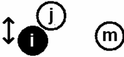
**Figure 4:** Mixing index determined with the neighbour distance method for the z-direction. Particle *j* is the closest partner for the highlighted particle *i*. Particle *m* has the least distance in the z-direction, but is not used as closest initial partner.
