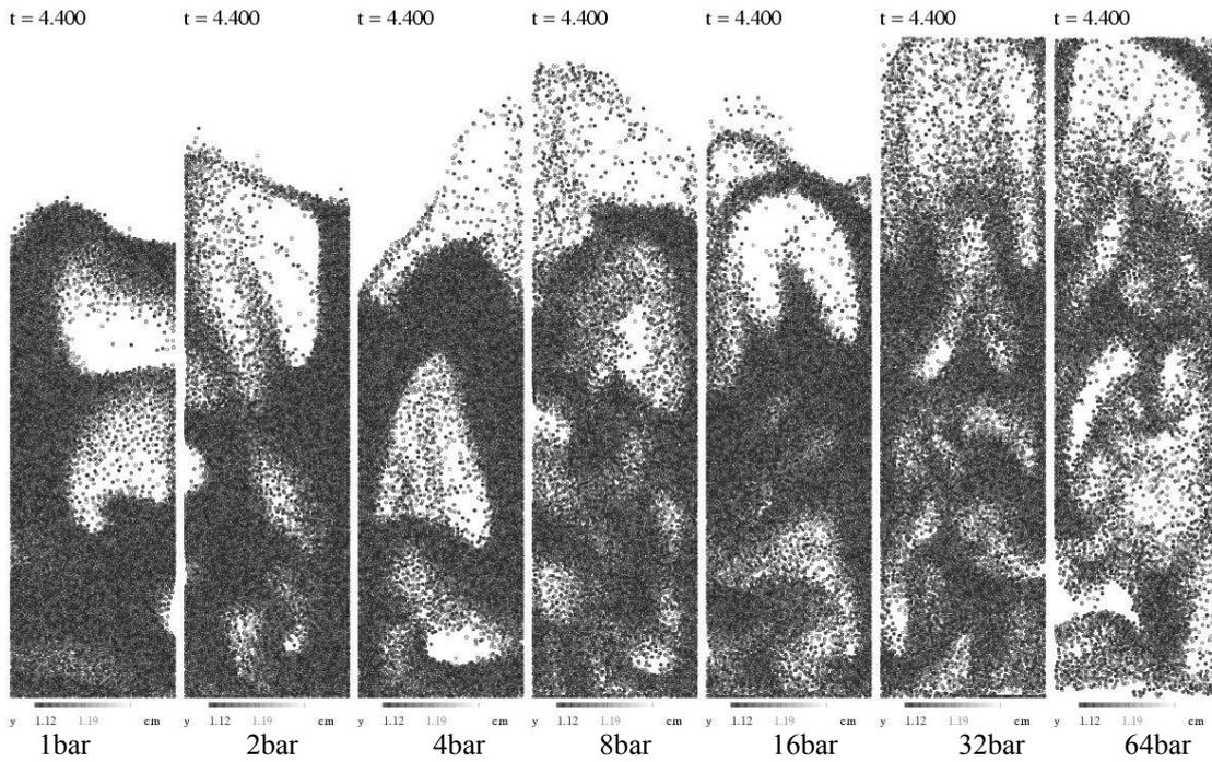
**Figure 8:** Snapshots of particle positions in a slice in the centre of the bed with a depth of one numerical grid cell at different operating pressures.
