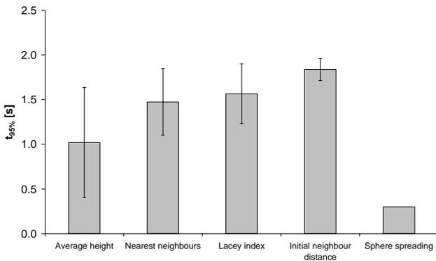
**Figure 9:** The 95% mixing time for all five methods for the simulation at 1 bar operating pressure. (Initially the top half of the particles were coloured black). The shown error margins are twice the standard deviation in the eight individual calculations of the 95% mixing time.
