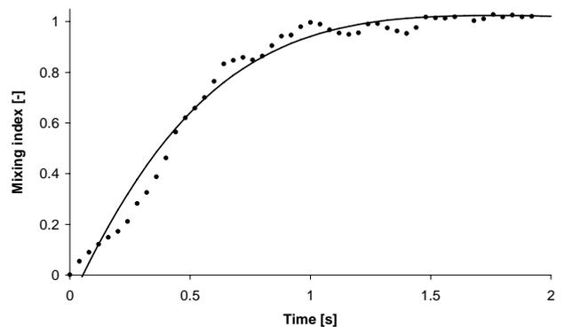
**Figure 6:** Lacey index fitted with a damped exponential function.
