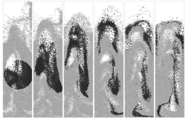
**Figure 5:** A slice in the middle of the fluidized bed is shown. Initially a sphere of particles is coloured black (left). After 0.2 seconds the sphere is spread over the bed (right).
