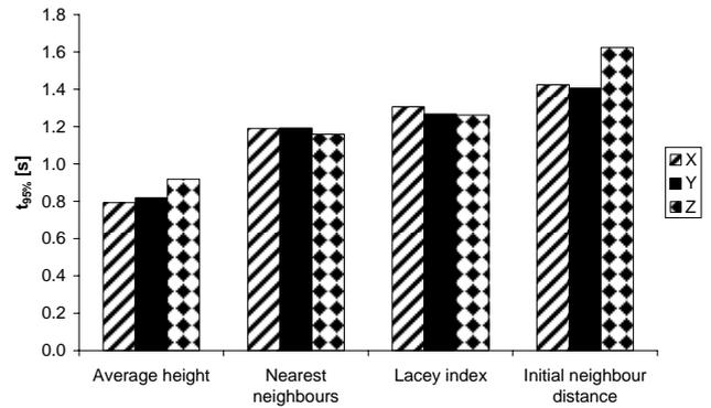
**Figure 12:** Mixing time for four mixing methods in vertical (z) and horizontal (x and y) directions for the simulation at 8 bar.
