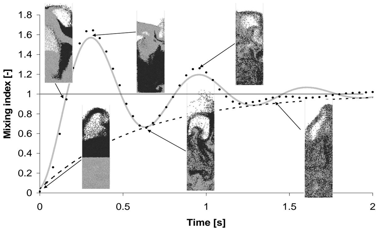
**Figure 7:** Mixing index versus time, resulting from simulations (•), a fit of the data using eq. 18 (—), and eq. 16 (---). Images of the particles present in a slice in the centre of the bed are shown as well.
