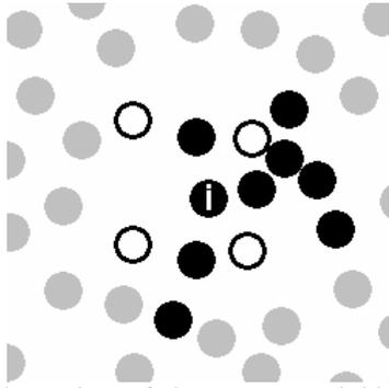
**Figure 1:** Illustration of the nearest neighbours method. For the highlighted particle (i) the twelve nearest neighbours are shown. Four of them are white and eight are coloured black. Particles that are located further away are coloured grey and are not taken into account for this particle.
