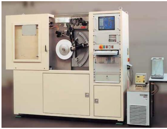
Fig. 2 Illustration and basic principle of LAT 100 to simulate WSR as a function of temperature.
