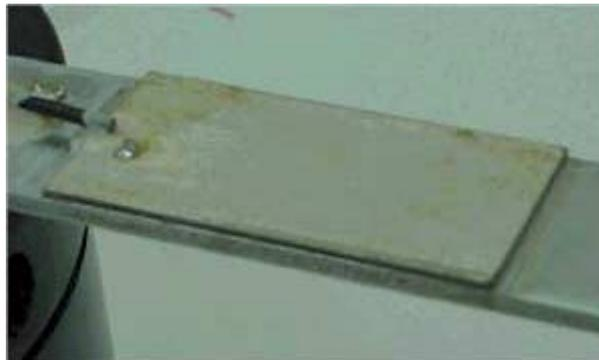
**Figure 1:** Piezoelectric patch bonded to a beam
