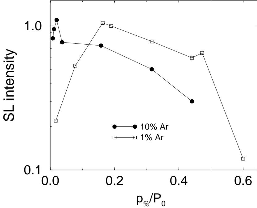
FIG. 5. SL intensity (normalized to air) from a SL bubble in water as a function of the gas mixture  $p_{\infty}/P_0$  for two different argon-nitrogen gas mixtures. The data are taken from figure 23 of Barber et al. [2].
