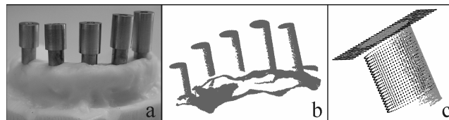
Fig. 3: Measurement of position of implants: (a) registration elements mounted upon implant replicas of work model, (b) point cloud of scanned elements, (c) fit of top plane and cylinder surface on identified points of a registration element.
