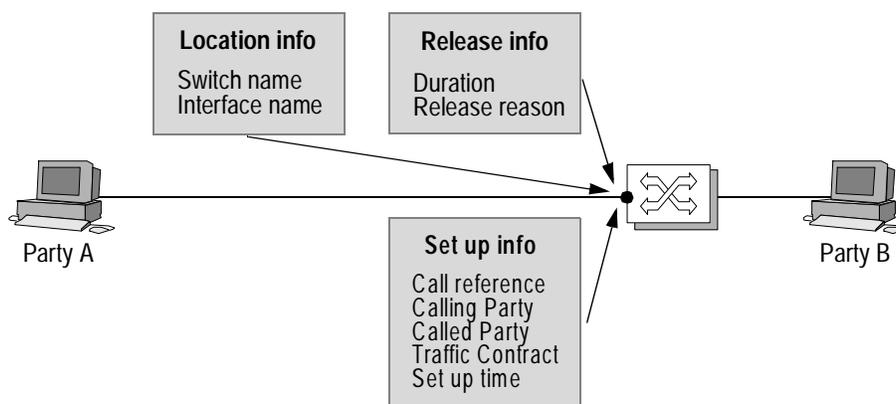
Figure 4: Usage Metering for a Connection
