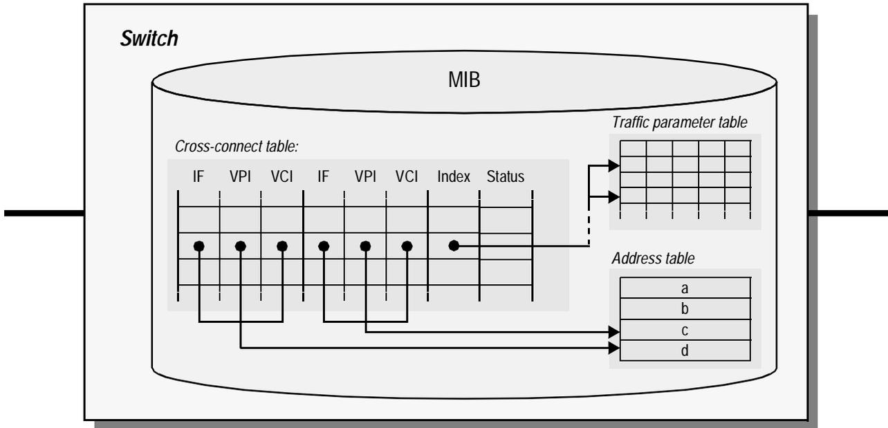
Figure 3: Aborting connections, based on IETF MIBs
