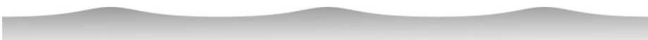
Figure 1.2: A periodic wave solution to the variational Boussinesq model (VBM), Eqs. (1.14) with a parabolic shape function (1.9) for the vertical flow structure. The mean water depth is 5 m, the wave height is 1.8 m and the period is 6 s.
