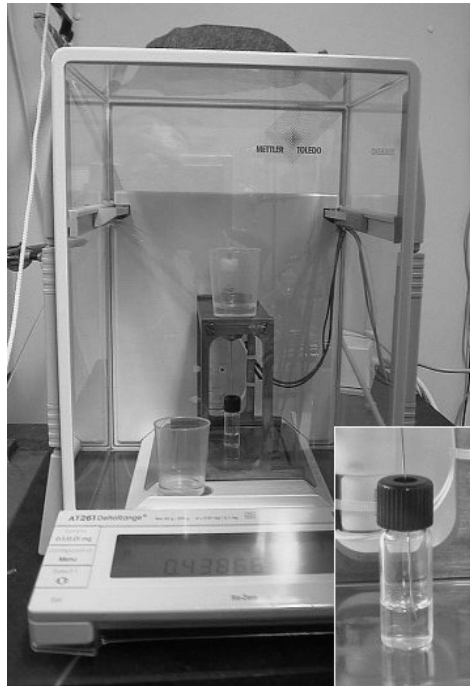
Figure 17 : The precision balance with the container. The inset shows the needle through which the pump discharges in the container.
