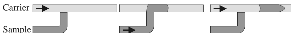
Figure 6: In a FIA system, the sample is injected into the carrier stream.
