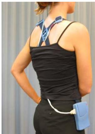
**Picture 1.1:** Myofeedback device consisting of a harness with dry surface electrodes and a sEMG storage and processing unit
