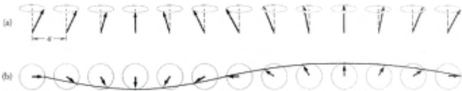
Figure 2.15: A 1-dimensional lattice of spins with a spin-wave, viewed in perspective (a) and from above (b). Taken from [69].
