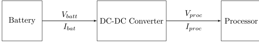
Figure 6.2: System level configuration of a single processor. V_{batt} ( I_{bat} ) and V_{proc} ( I_{proc} ) represents the voltage (current) of the battery and processor respectively.
