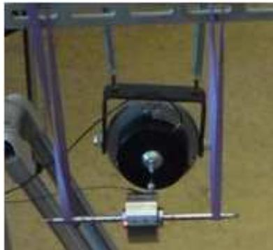
Figure 8.3: Modal analysis of the free rotor
